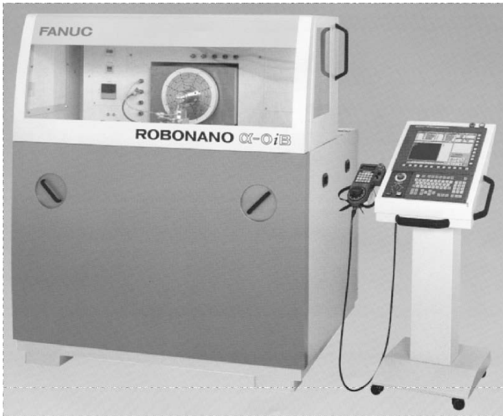
Figure 10.27. FANUC RoboNANO \alpha -OiB super precision micro machining center, from FANUC 239 .
