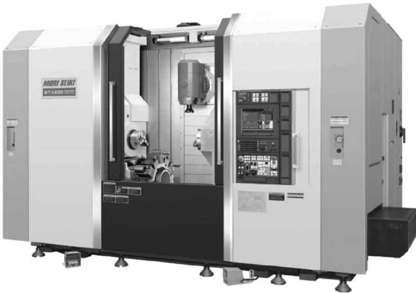
Figure 5.29. Mori Seiki “mill-turn” machine operating area enclosure open for access, courtesy of Mori Seiki.
