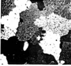
a. Equiaxed grains in ingot of material
